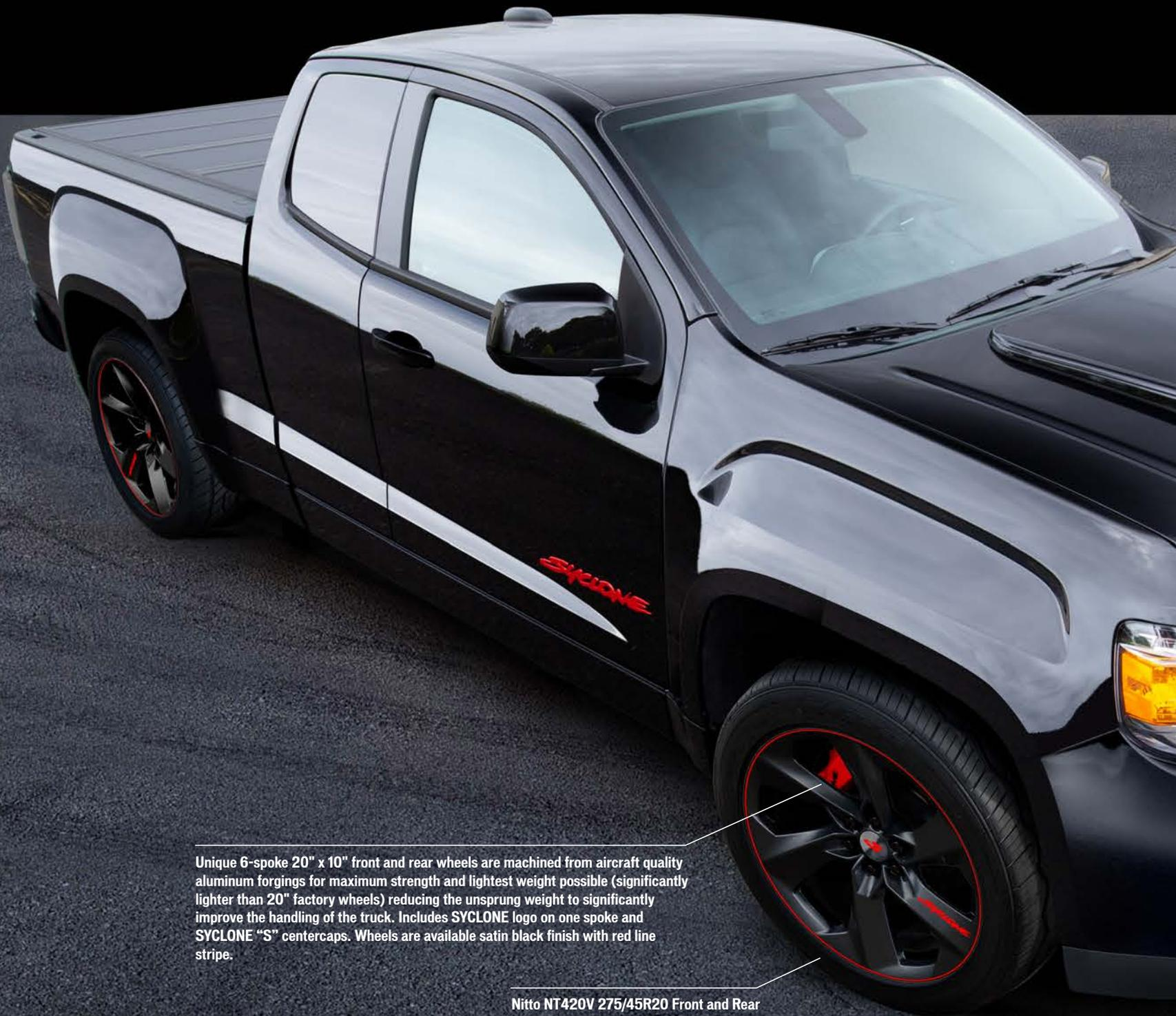
Unique 6-spoke 20" x 10" front and rear wheels are machined from aircraft quality aluminum forgings for maximum strength and lightest weight possible (significantly lighter than 20" factory wheels) reducing the unsprung weight to significantly improve the handling of the truck. Includes SYCLONE logo on one spoke and SYCLONE "S" centercaps. Wheels are available satin black finish with red line stripe.
