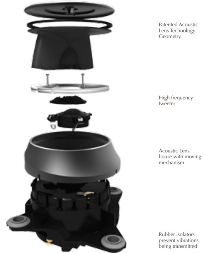
Patented Acoustic Lens Technology Geometry
