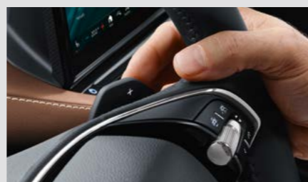
2-spoke leather heated multi-function steering wheel with paddles for recuperation level selection
