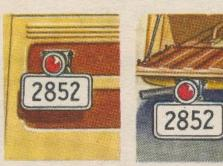
TAIL LIGHT and license-plate holder swivels to position shown above at right when tailgate is left down to haul bulky objects.
