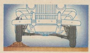
STABILIZED RIDING and easier steering result from Willys-Overland's new front-wheel suspension and rubber-insert springs. Diagram at left shows how one wheel goes over a road obstruction, maintaining a nearly vertical plane and with minimum body tilt. The result is an easier ride, more tire economy and better steering control.
