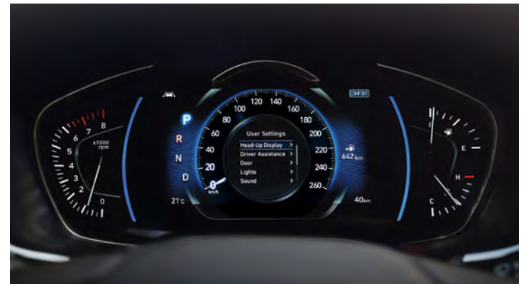
Available electro-luminescent gauge cluster with 7.0" supervision LCD trip computer
