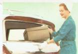
ROLL-DOWN REAR WINDOW on 4-door station wagons disappears into tailgate. On 2-door wagon models, the tailgate is a fifth door that swings wide open.
