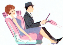
LOUNGE-TILT SEAT* offers the restful comfort of a contoured lounge chair. Seat cushion adjusts upward for knee height, seat-back adjusts to reclining positions, headrest adjusts for comfort and safety, seat glides back and forth. Available for front passenger and driver.
