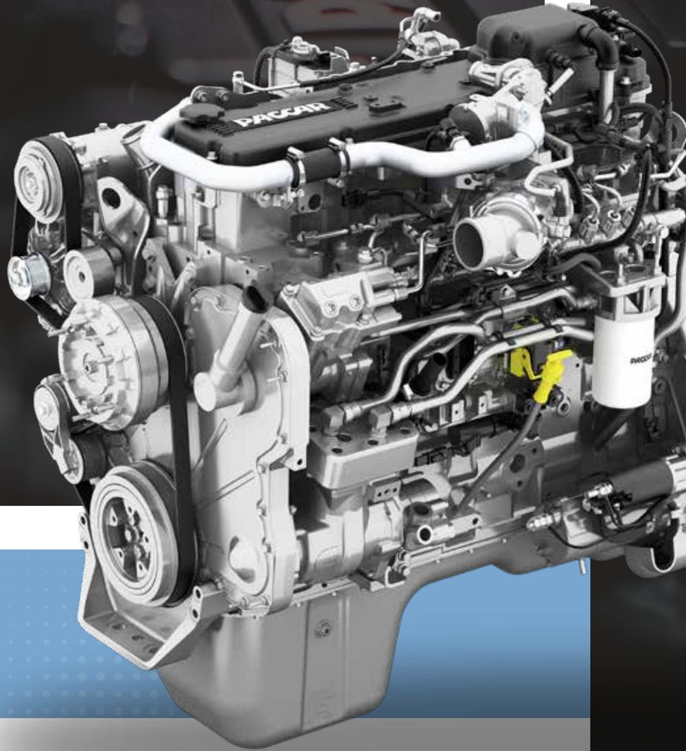
The 8.9-liter PACCAR PX-9 engine has one of the highest power-to-weight ratios in its class, and will move heavy payloads without hesitation.
