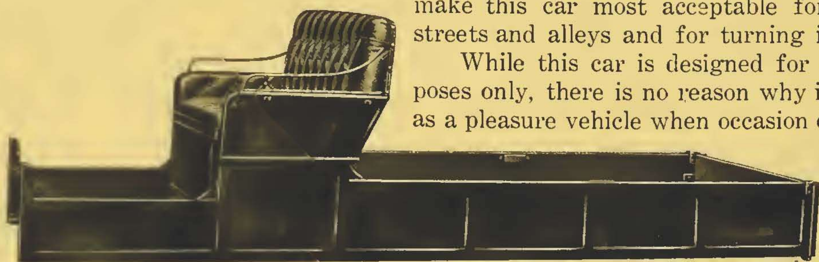
This box can be placed upon the chassis of the auto buggy, making a business vehicle
