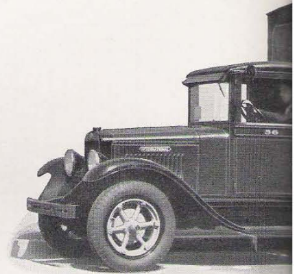
Van bodies of all types are readily adapted to the Model A-2. This type of body combination is particularly popular.
