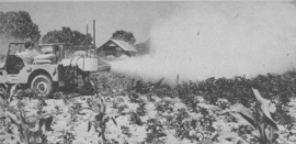
With a duster mounted in the "Jeep" and powered by the "Jeep" power take-off, you can cover your potatoes and other crops in a hurry. Note the extra sacks the "Jeep" carries along in the truck bed.
