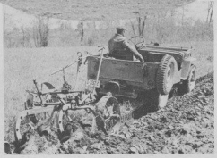
With 4-wheel drive and in "low low" gear, the "Jeep" is rated at 1,200 pounds of continuous draw bar pull, with reserve power for extra loads. In a 400-acre field test, the "Jeep" pulled a double-bottom 12-inch plow, plowing about an acre an hour with fuel consumption of 1½ gallons per hour.
