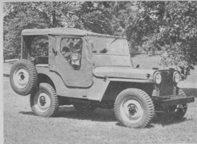
Ready for Winter—"Jeep" with front and rear top, and door curtains. Side and rear curtains are removable, as shown above.
