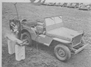
Portable arc-welding equipment with its own "Jeep" - power-driven generator makes possible arc-welding far from the power lines. Another job for the Universal "Jeep" in industry and on the farm.
