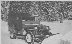
Here's still another job for the Universal "Jeep" - clearing roads and streets with a special snow blade. The power of 4-wheel-drive gives the "Jeep" the push to get this job done fast for street departments and industry.
