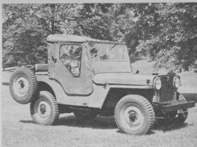
The Universal "Jeep" has added convenience and comfort for driver and passengers—improved springs and shock absorbers, cushioned spring seats, etc. Removable front top with curtained doors and rear curtains is optional accessory.
