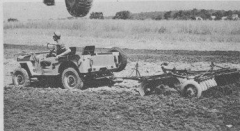
(Above) The Universal "Jeep" pulls a 7-ft. tandem disc on a Michigan farm. With tractor speeds of 2 to 7½ miles per hour, the "Jeep" works fast and economically.
