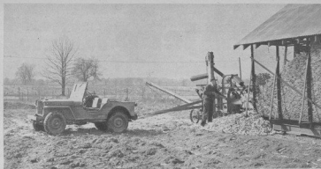
When you "Get a Jeep", you get four vehicles in one—truck, tractor, runabout and mobile unit. Above, a "Jeep" with the special power take-off delivers even power to a corn sheller. The Willys "Jeep" Engine that supplies the power is the same mighty engine, war-tested in military "Jeeps" in every climate on the globe.
