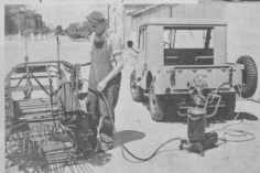
Wherever power is needed, the "Jeep" will take it. This pressure lubricator, carried in the "Jeep" and powered by the power take-off saves hours in bringing equipment to a central point for lubrication and repairs.
