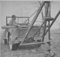
The "Jeep" with power take-off delivers the power where you need it, in the barn yard or to the toughest spots. Here the versatile "Jeep" goes down the fence line powering a post-hole auger, getting the job done in double-quick time. Note the driver's clear vision of the auger.
