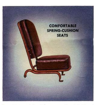
Easy-riding seats built with new-type springs, hair felt and cotton padding. Upholstered in durable simulated leather. Modern tubular-steel frames with chrome foot rests. All except driver's seat can be removed.
