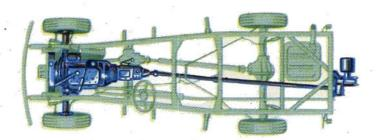
**CHASSIS** of the sensational 4-wheel-drive 'Jeep' Truck, showing two live axles that give tractive effort on all wheels. Note transfer case, back of transmission, which permits selection of 2-wheel drive, or 4-wheel drive with 6 speeds forward, 2 reverse. Optional power take-off is operated by shaft from rear of transfer case.
