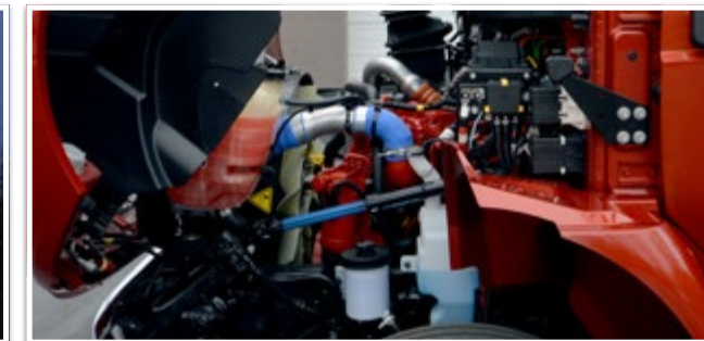
Key fluid reservoirs are translucent for quick inspection and many of the caps are tethered, saving time and frustration from dropped or lost caps
