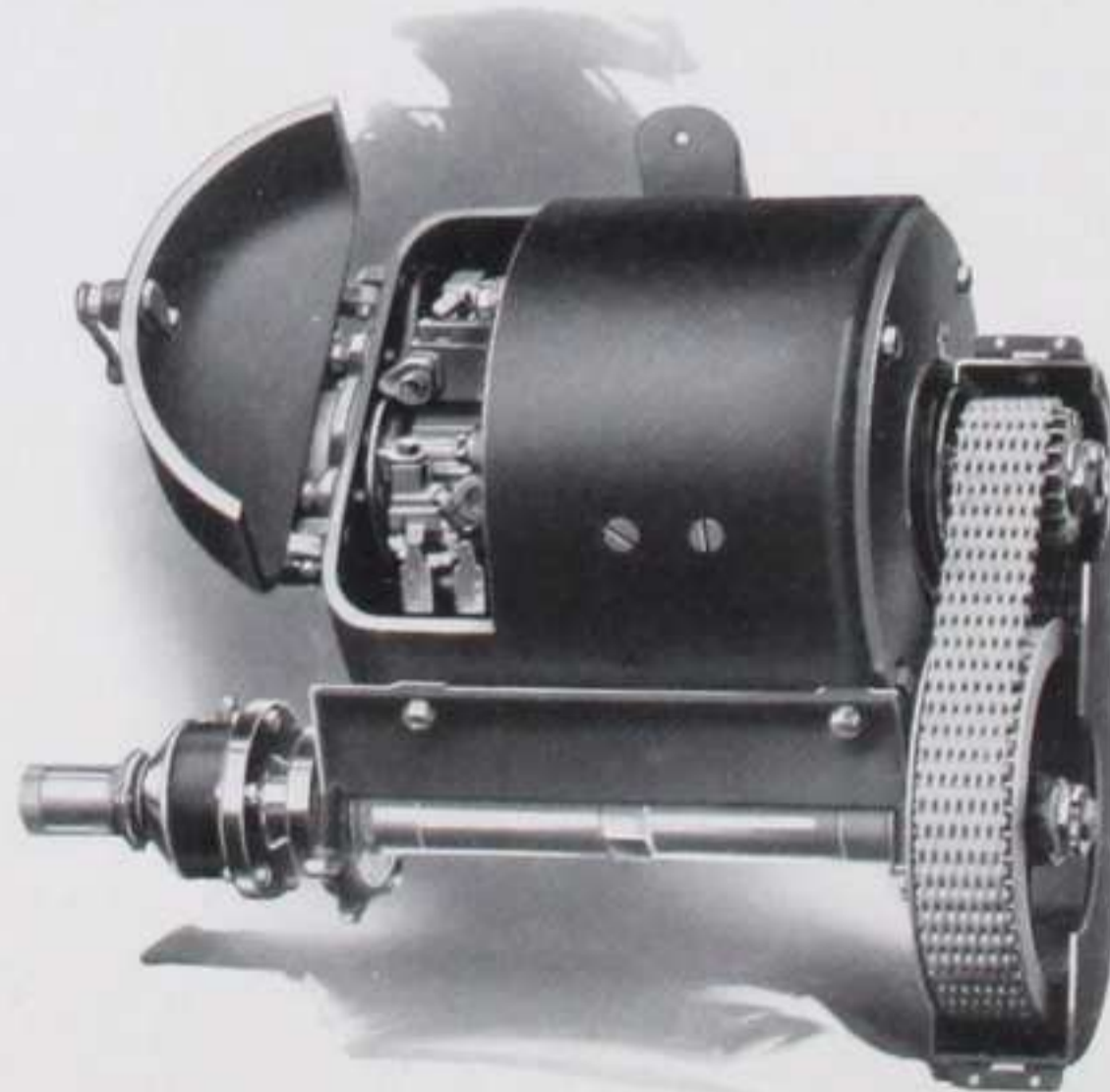
Baker Electric Motor — Silent Chain Reduction and Countershaft
