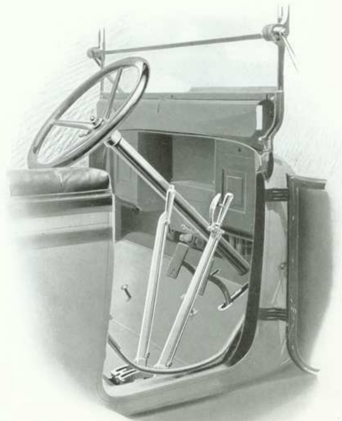
Control Levers are inside with ample clearance
