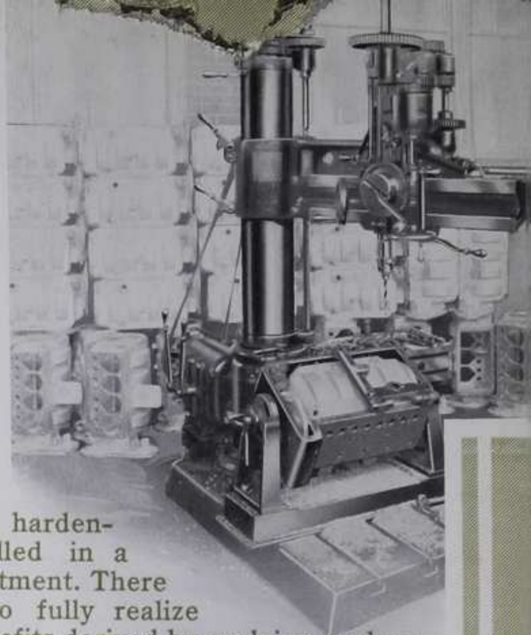
RADIAL DRILL, DRILLING CRANK CASE BY USE OF JIG All holes are drilled in casting before removed from jig, insuring uniformity of parts and economy of manufacture.
