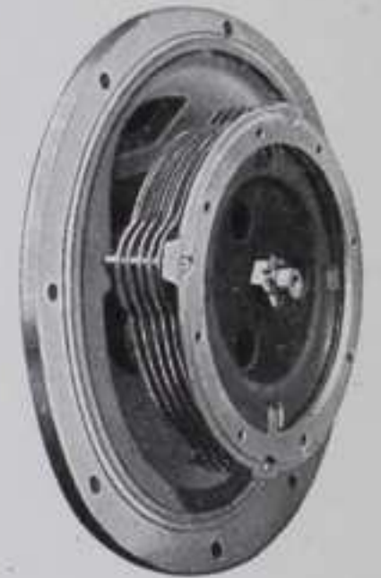
MULTIPLE DISC CLUTCH Used on Models 38 and 40
