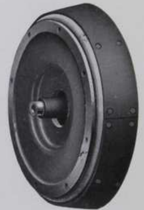
CONE CLUTCH Diameter 13\frac{3}{4} ". Face 2\frac{3}{8} ". Used on models 33, 34 and 35
