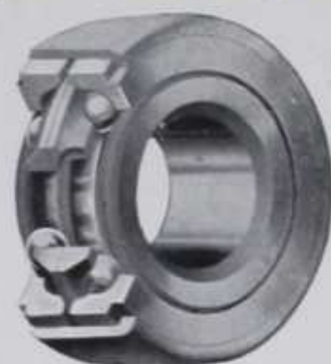
NEW DEPARTURE DOUBLE-ROW ANNULAR BALL BEARING Outside Diameter, 3\frac{3}{8} ". Diameter of balls, \frac{1}{2} ". Used directly back of main driving pinion in rear axle.
