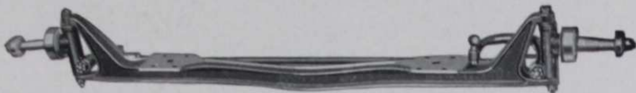
Front axle with 100% thrust genuine annular ball bearings used in front wheels. Note unusual "heft" and sturdiness of the forging and steering knuckles.
