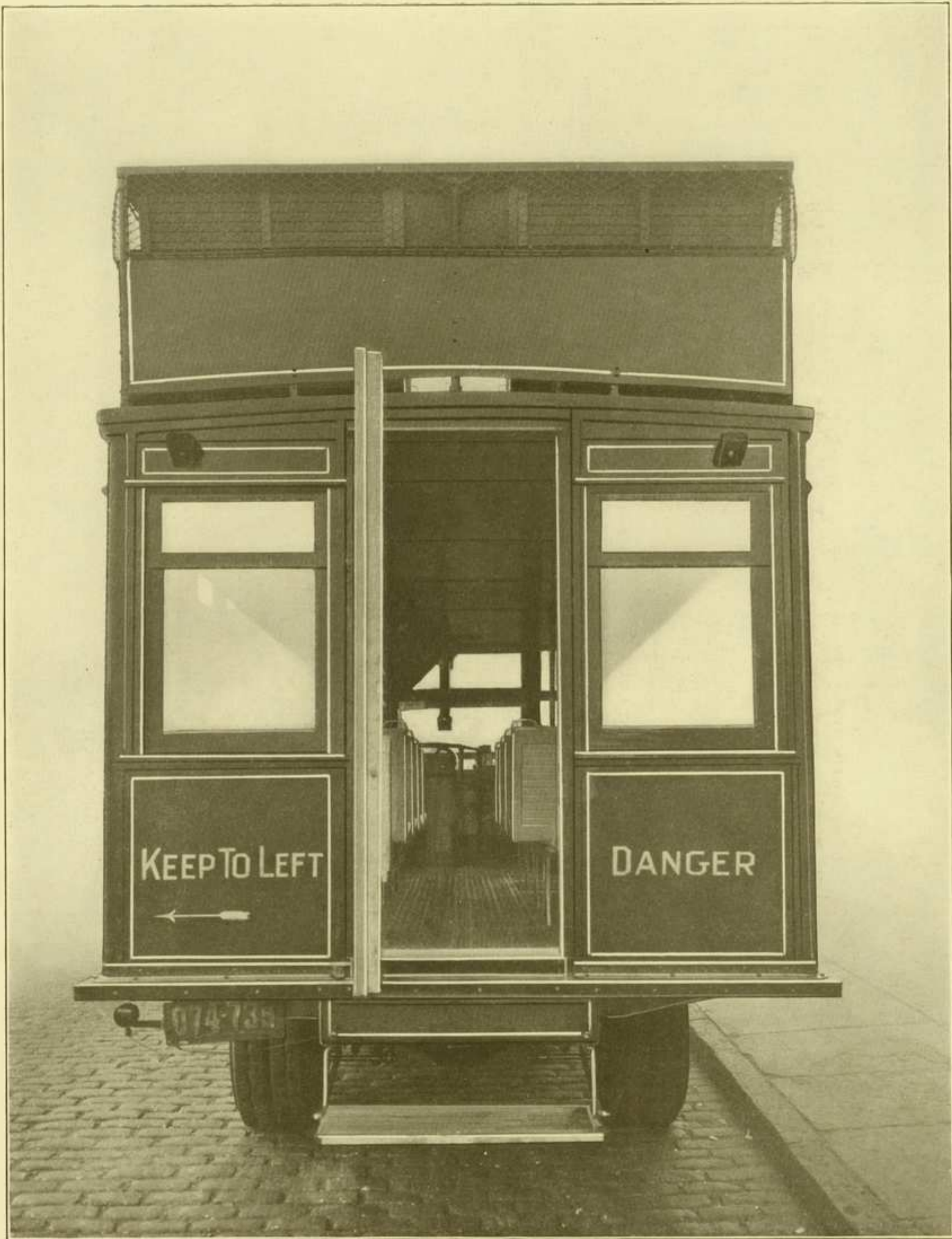
Exterior view of Leindorf One Man Double Deck Safety Bus, showing emergency exit door open and step dropped automatically by the opening of the door—IMPORTANT—The majority of transportation experts now insist that a rear emergency exit door is absolutely necessary for safety in front entrance buses—The majority of front entrance single deck buses are still built and operated without them.
