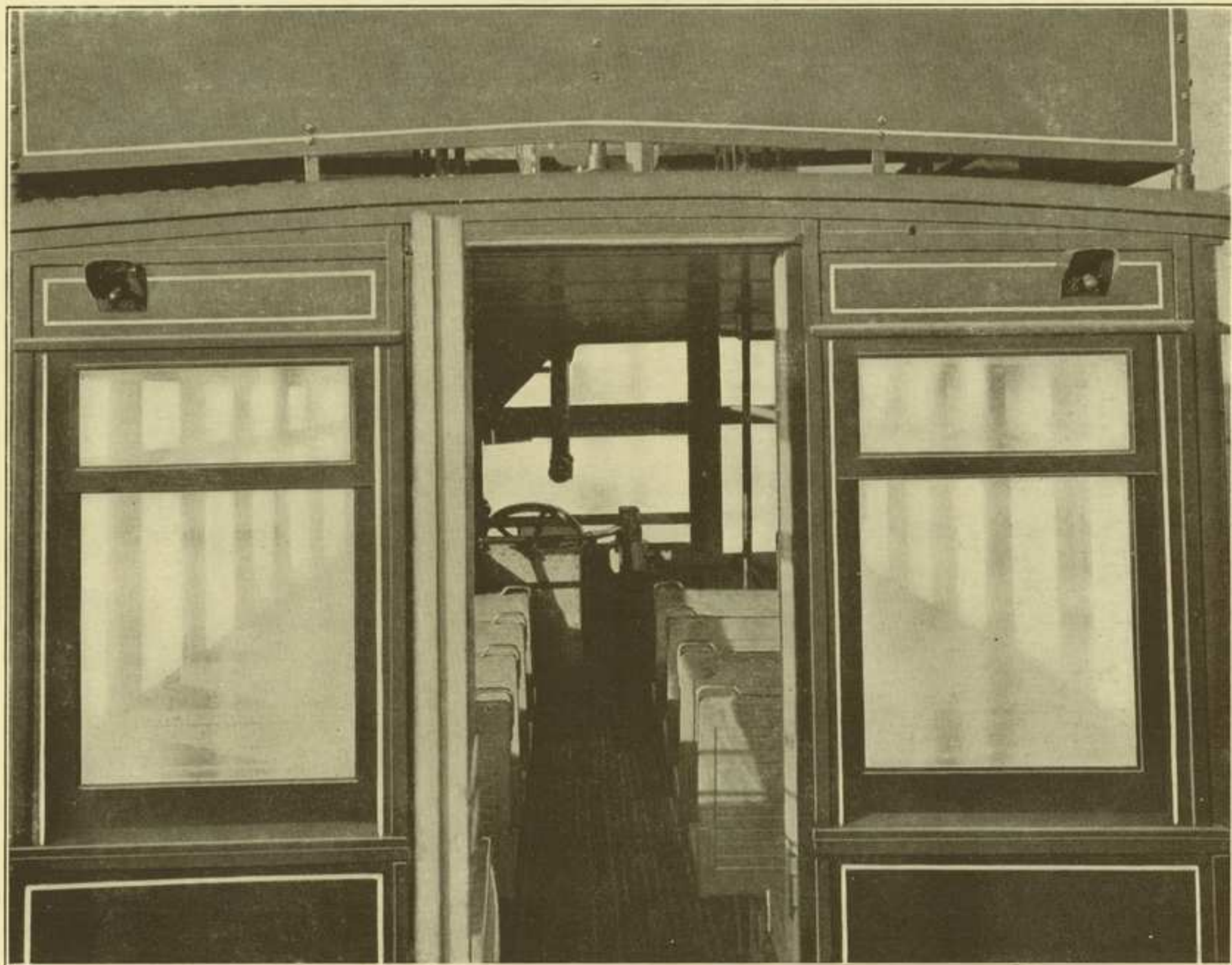
Interior view through opened emergency exit, showing safe aisle space for standees—Note space at top of rear for route designations or advertising.
