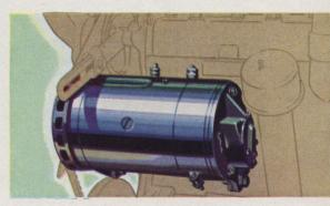
The big generator, driven by the fan belt, is air-cooled for greater charging capacity and produces ample current for sure starting and all electrical accessories you may add.
