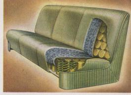
Comfort and durability are built into the Kaiser Special seat cushions. Coil springs are topped with soft padding, under upholstery,
