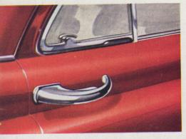
Only a slight squeeze on the "trigger" control of each outside door handle suffices to release the lock. The handle does not turn.
