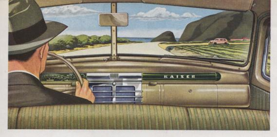
An exceptionally wide windshield increases the driver's side vision as well as providing a better view of the road ahead. Forward vision is also improved by the design of the hood which permits the driver to see the road close to the car. There is no hood ornament.
