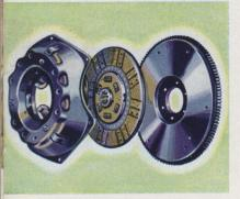
Clutch action is smooth and positive. Mechanism is a 9¼-inch-diameter plate and a sealed ball release bearing.
