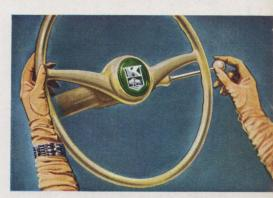
The modern steering wheel of the Kaiser Special has no vertical spoke to impede the driver's view of the speedometer and gauges.
