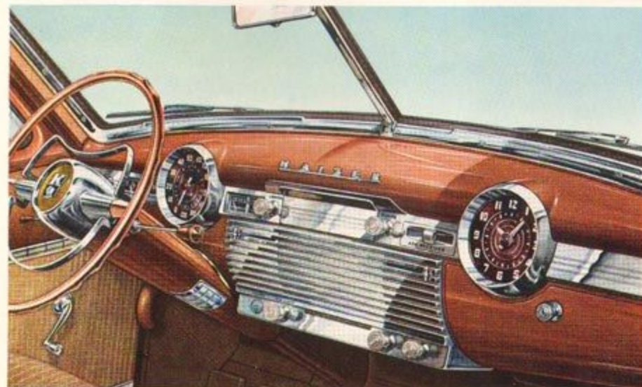
MODERN DESIGN FOR DRIVING! Modern steering wheel unit and instrument panel make driving easier, provide obstruction-free vision of highly readable speedometer and gauges. Indirect illumination is regulated for degree of brightness. Map light located on steering column shield.
