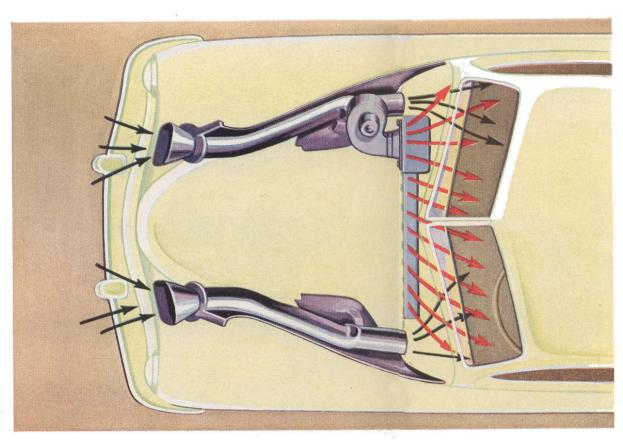
An integral part of the Kaiser air conditioner is the built-in defroster unit which permits windshield and windows to stay clear of fog and steam under virtually all conditions.
