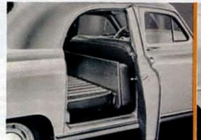
There are several things to note in this photograph of the Traveler. First, the floor is smooth and flat when the rear seat is folded. Second, the front floor is supported by an angle iron on the bottom of the front seat which extends full width. Third, the bottom of the seat, forming the end of the cargo hold, is of plywood.
