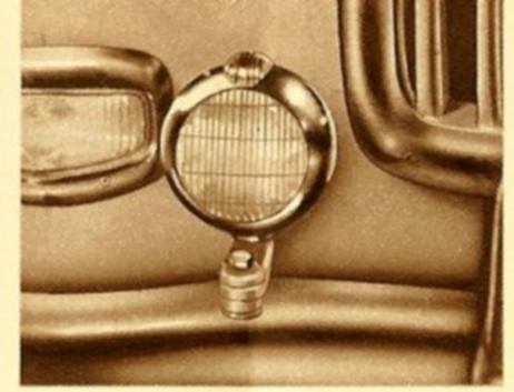
weather driving. These sealed-beam units assure fixed focus, trouble-free light for maximum visibility in fog, sleet, rain or snow.
