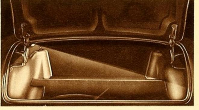
NASH TRUNK LIGHT. Gives uniform illumination throughout trunk compartment—a real convenience when loading luggage or removing spare tire at night.
