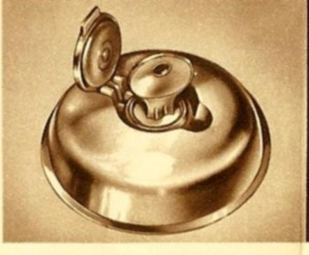
fuel thefts on your Rambler. Turn key and cap lifts off. Remove key and snap the cap back over the filler neck. Cap locks automatically when in place.
