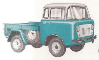
"JEEP' FC-150 TRUCK puts maximum payload on minimum wheelbase. Has shorter turn radius for higher maneuverability. Wide window visibility. F-Head "Hurricane" engine gives 4-cylinder economy.
