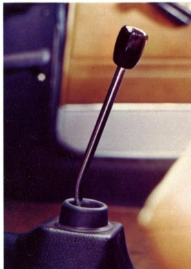
Four speed all synchromesh gearbox with floor mounted stick shift
