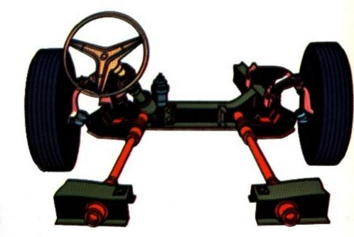
Torsion bar suspension, long a feature of Plymouth engineering, has proved an exceptional replacement for conventional front-end coil springs. Plymouth's torsion bars actually twist and flex to rid your car of road shock and to smooth out a bumpy road.
