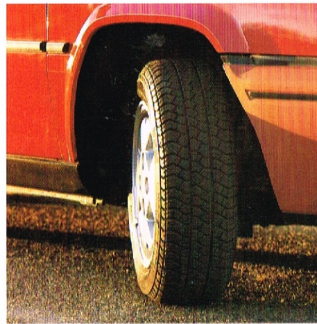
Even the wheel arches have moulded liners to prevent damage from flying stones. (above).
