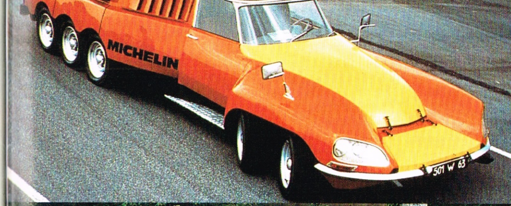
The 10-wheeled Citroën developed by Michelin to test tyres
