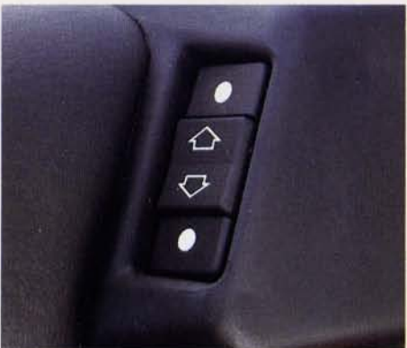
Driver's electric window has one-touch open and closing as well as conventional operation.
