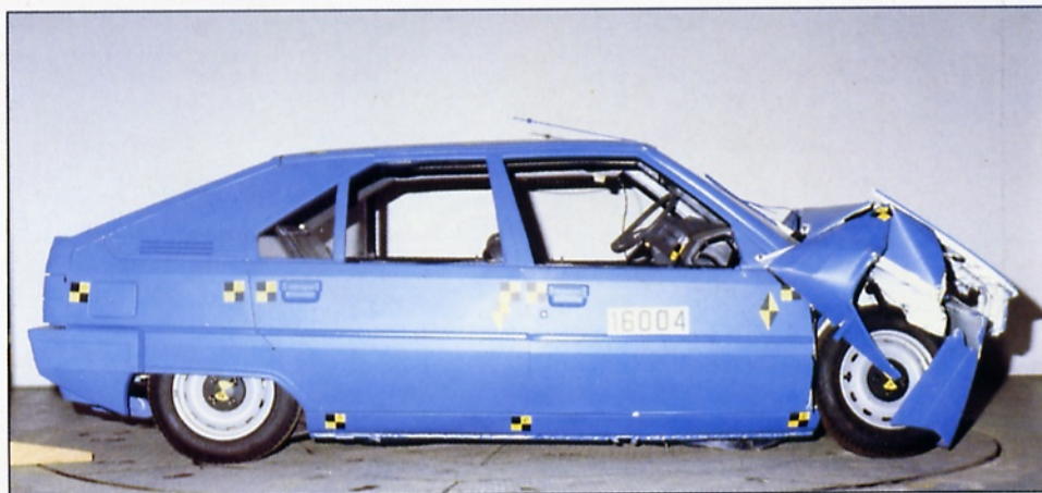
The bodyshell design and choice of materials ensure that in a serious collision the BX's passenger compartment retains its integrity while the front of the car is designed to crumple in a controlled manner, reducing the force of the impact.
