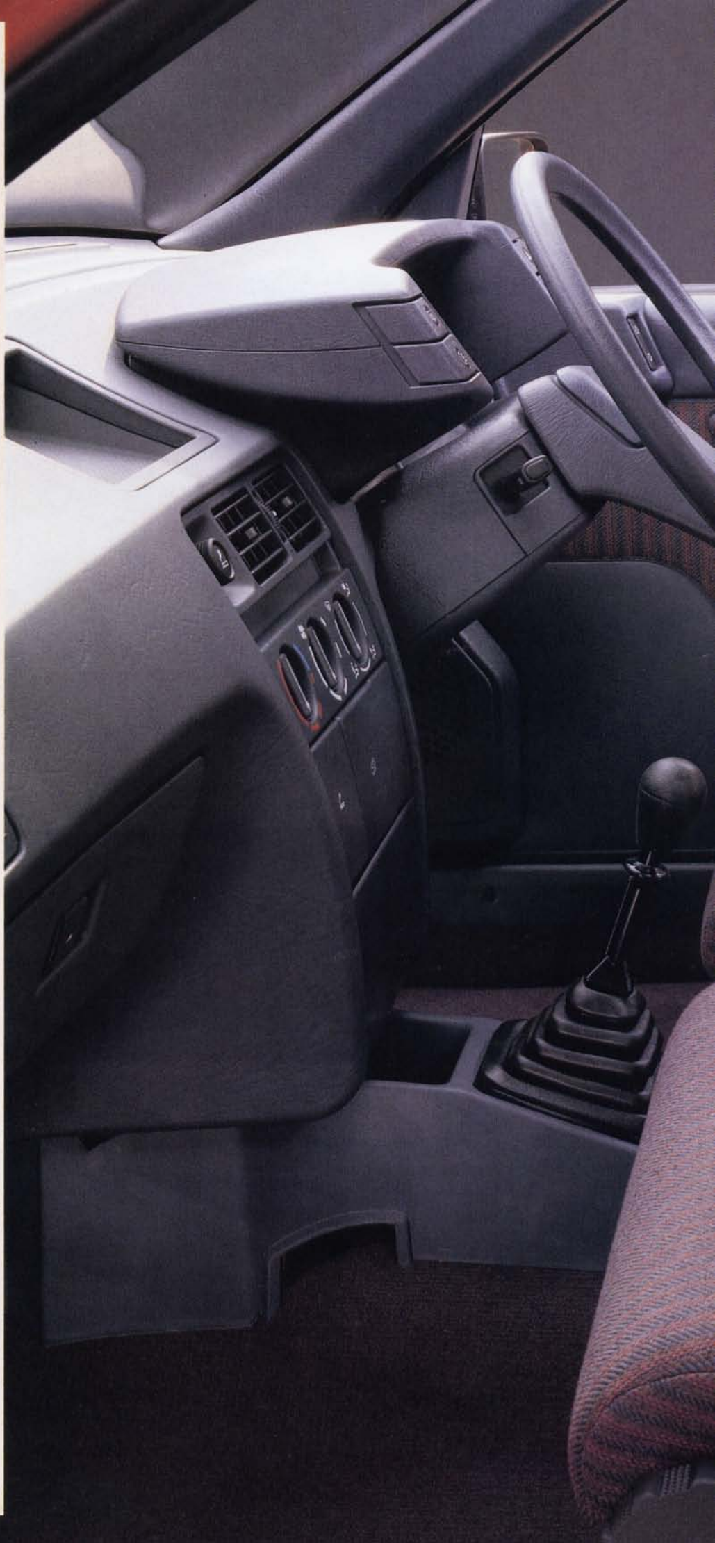
Single spoke steering wheel ensures instrument visibility, and collapses safely in a major impact.
