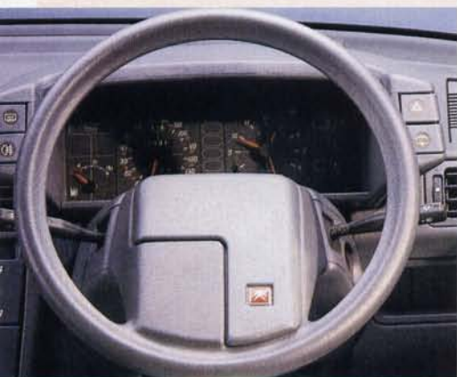
Single spoke steering wheel ensures instrument visibility, and collapses safely in a major impact.
