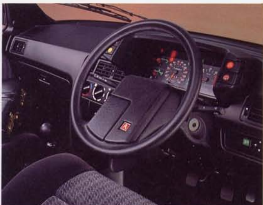
Steering wheel design ensures instrument visibility and collapses safely in a major impact.
