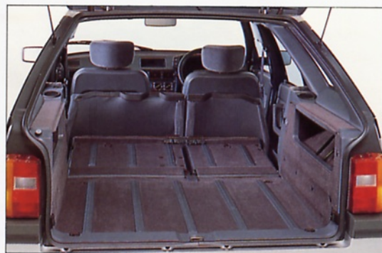
A flat unobstructed load space of 63.7 cu ft with rear seats folded.
