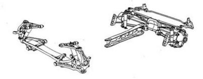
All Corvettes have a four-wheel independent front and rear suspension. The front is comprised of parallel forged-aluminum upper and lower control arms and steering knuckle, glass-epoxy transverse monoleaf spring and a steel anti-roll bar.
