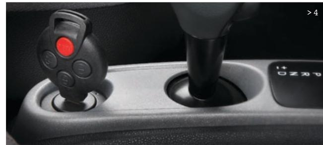
> **4 4-button smart key including panic button:** For highly convenient central locking and unlocking of your pure by remote control. Including remote rear window release (pure and passion coupe), roof release (passion cabriolet) and panic button.
