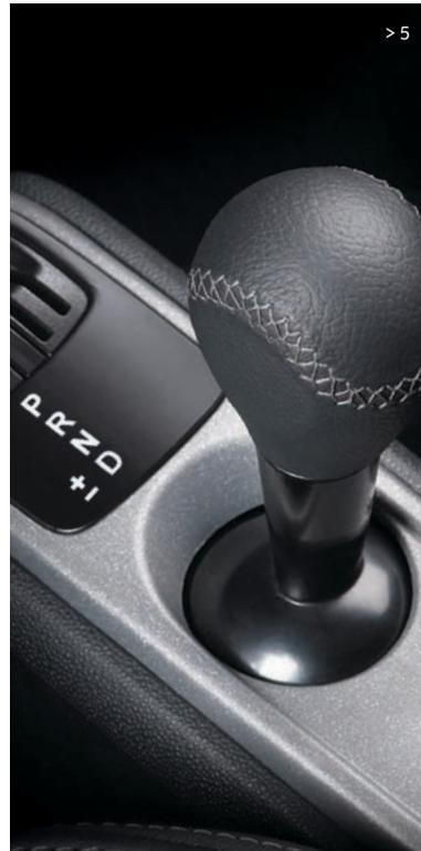
> **5 5-speed automated manual transmission:** Changing gears has never been simpler – a gentle tap on the leather wrapped gearshift lever changes up and down or simply choose "D" for the automated gear change. Includes kickdown function.
