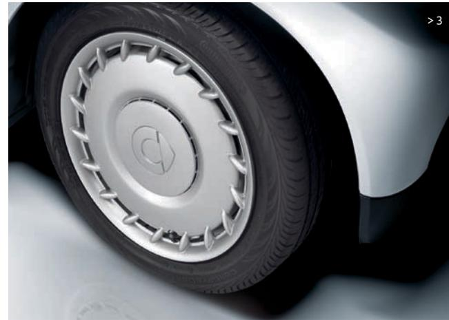
> **3 Steel wheels (15") with smart wheel covers:** Sturdy and functional. Fitted with 155/60 R 15 tires at the front and 175/55 R 15 tires at the rear.
