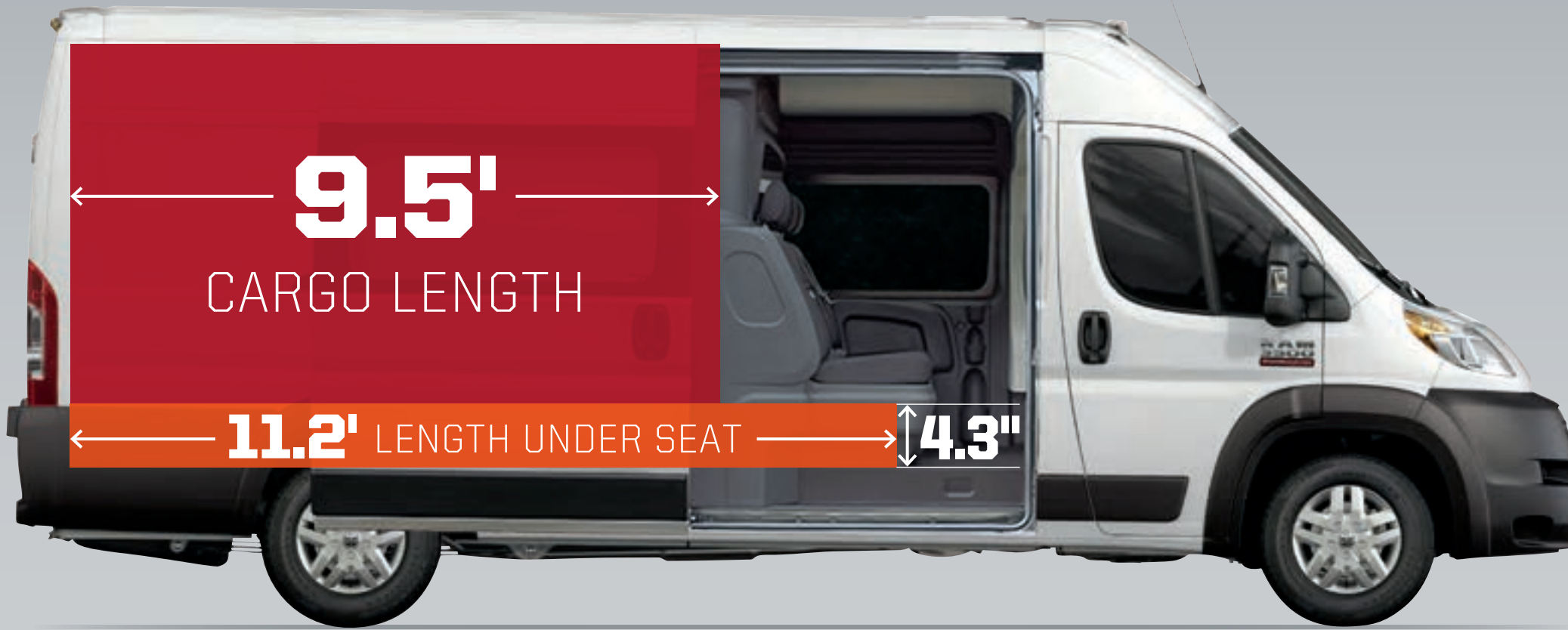
159-inch wheelbase, extended with Crew Van Package
