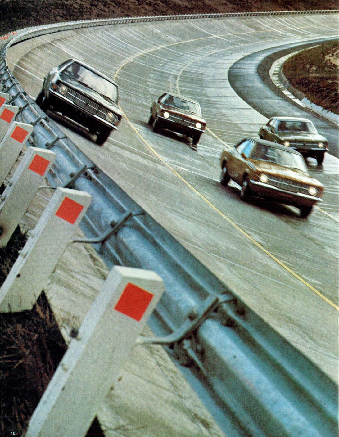
Opposite: Durability testing, constant speed circuit at Ford's You Yangs Proving Ground.
