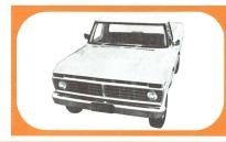
Independent suspension by twin I beam and coil springs Capacity 1590 kg (3500 lb)
