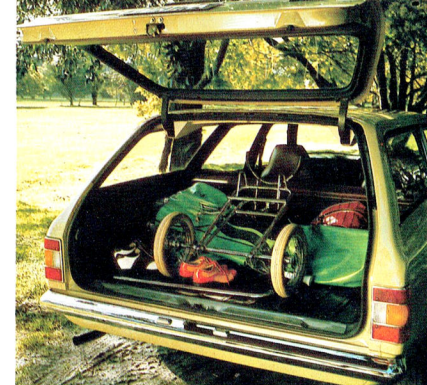
One-piece counter-balanced rear door — 1.81m 2 load space
