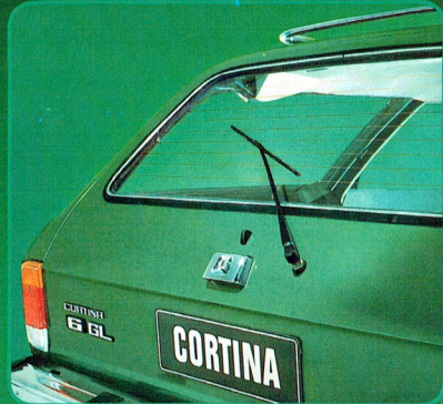
Cortina GL Wagon features a rear-window washer, wiper and demister.
