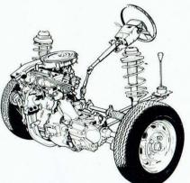
To begin with, being a front wheel drive, the major mechanicals are mounted sideways or transversely and incorporate engine, clutch, transmission and final drive. This compact unit fits neatly across the engine compartment, leaving space for easy access without taking up a great deal of the car
