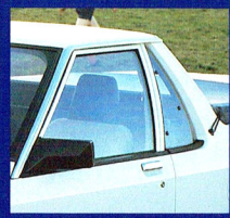
Illustrated: Falcon GL Ute showing opening side air extraction windows.
