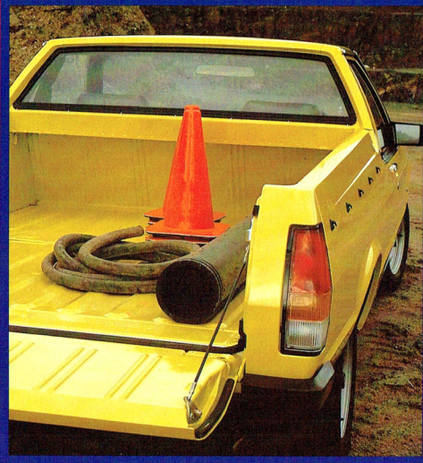
Illustrated: Ford Falcon Ute. The business end. Three-quarter tonne capacity. Heavy gauge steel floor load area with ribbing for extra strength and easy loading/unloading. Double panelled sides in load area.
