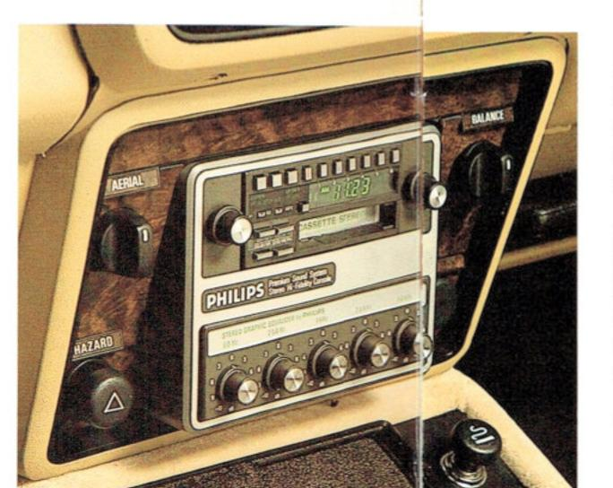
The tape deck is of high specification. It has a ceramic playback head and a Dolby\* noise reduction system to provide excellent sound reproduction. Designed for quiet opera-tion, its refinements include a muting circuit on fast-forward and rewind modes.
