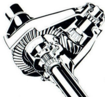
Bronco is equipped with rear Limited Slip Differential (LSD)
