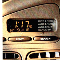
▲ The trip computer supplies data relating to speed and fuel consumption. It also includes an 'overspeed' function that warns you if you exceed a pre-set speed.
