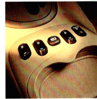
▲ The centre console houses the controls for Fairmont's front and rear power windows.
