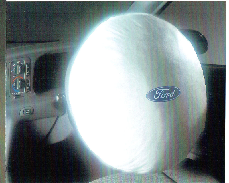
▲ The driver airbag is located behind a panel in the centre of the steering wheel.
