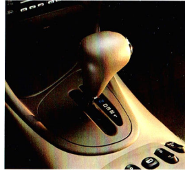
▶ The smooth and versatile Australian-made four-speed electronically controlled automatic transmission produces outstanding fuel economy with quiet operation. Fuel-saving features include a 'normal/economy' switch changeable by the driver to suit driving conditions and a torque converter with 'lock-up clutch' for third and fourth gears.
