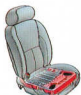
Taurus Ghia seats are designed to prevent the tendency of occupants to slide down and under their seat belts in the event of a sudden stop.
