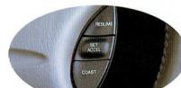
Cruise control makes long trips more relaxing. "Tap up or down" adjusts speed by small increments.
