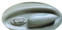
Front driver's seat has power operation for adjustments to fore and aft position, tilt and height.
