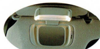
When the engine is switched off, a battery saver switches off the interior lights after 40 minutes should a door be left ajar.
