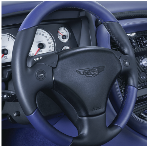
Touchtronic transmission – steering wheel controls and gear shift.
