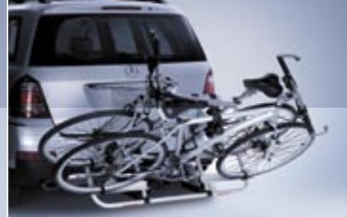
*The laden bicycle rack can be pivoted downwards, allowing the rear hatch to be opened*
