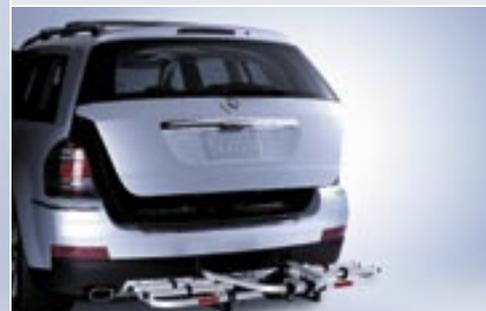
*When rack is unladen, simply fold down the vertical bar to gain access to the rear hatch*
