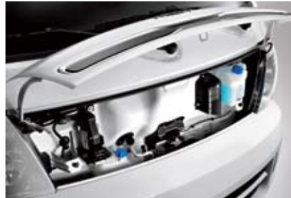
Front open panel : Allows you to easily check fluid levels and refill when necessary
