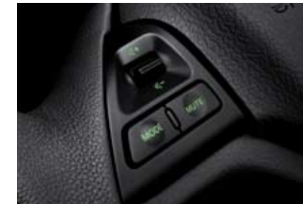
Steering wheel audio remote : Allows you to safely control a number of audio system functions without taking your eyes off the road
