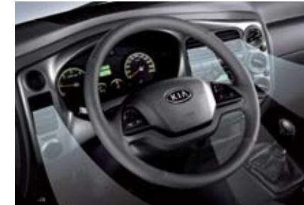
Heater : Rapidly warms the cabin on chilly days thanks to four separate vents
