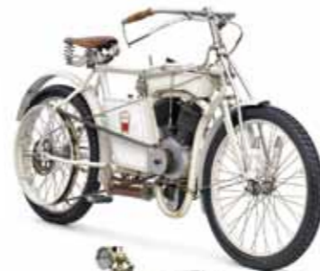
L&K type CCD Slavia motorcycle (1906) The factory's most popular two-cylinder motorcycle. 675 units were produced between 1904-1907
