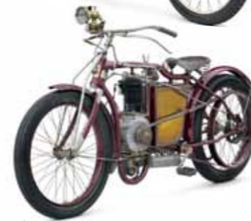
L&K type L motorcycle (1904) A sporting model with a lowered frame in the seat area.
