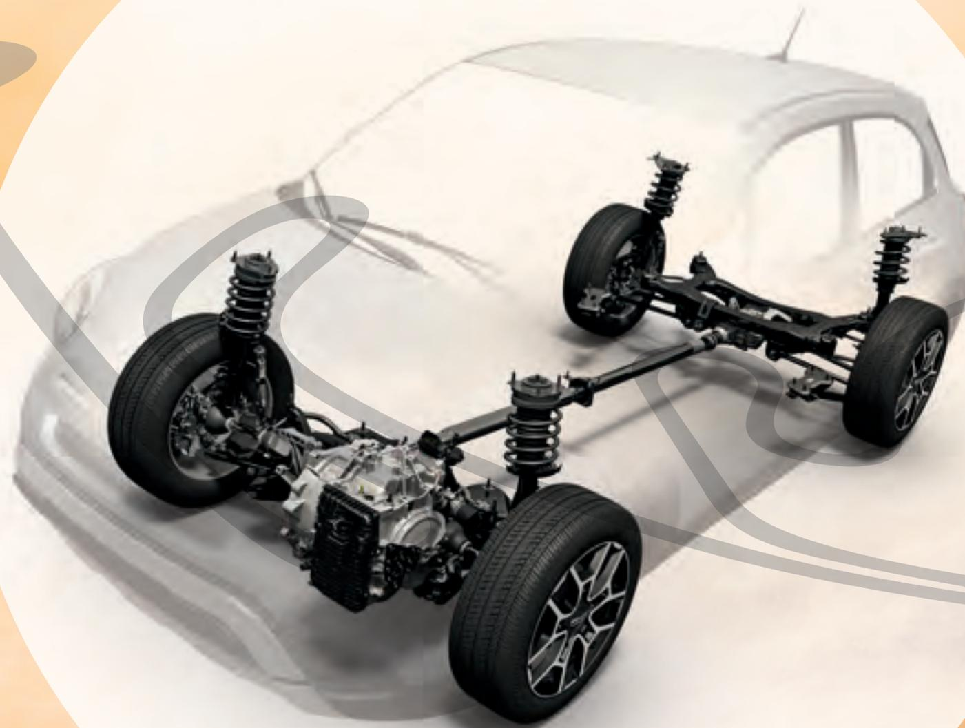
The FIAT® 500X also features KONI® Frequency Selective Damping (FSD) front and rear shock absorber technology to deliver impressive roadholding and handling characteristics. The KONI FSD system actively filters out inputs from uneven road surfaces and adjusts for comfort and smoothness while maintaining excellent ride control.
