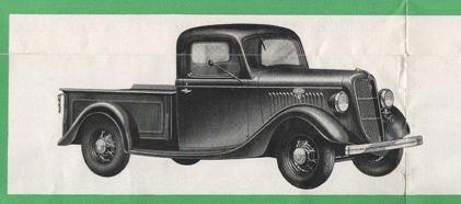
FORD V-8 UTILITY MODEL 50 — An outstanding new model available as chassis with cab, ready to be fitted with required body. Illustration shows unit complete with delivery body. Adaptable to all classes of utility service, this model will interest town and country users who require efficient, economical performance combined with maximum carrying capacity. Auxiliary rear springs optional equipment.
