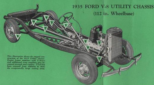
NEW FRONT-END CONSTRUCTION - Front spring and engine moved forward. Greater proportion of chassis length available for load space. Load centre moved forward, permitting better weight distribution. Front spring is longer. Increased front-end stability.
