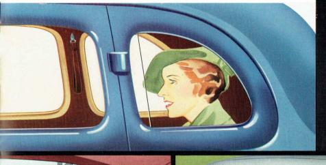
A Complete Built-in System of All-weather Ventilation: Improved clear-vision window ventilation—no pillars to cause "blind-spots" for the driver. Wide cowl ventilator with screen. A windscreen that opens.
