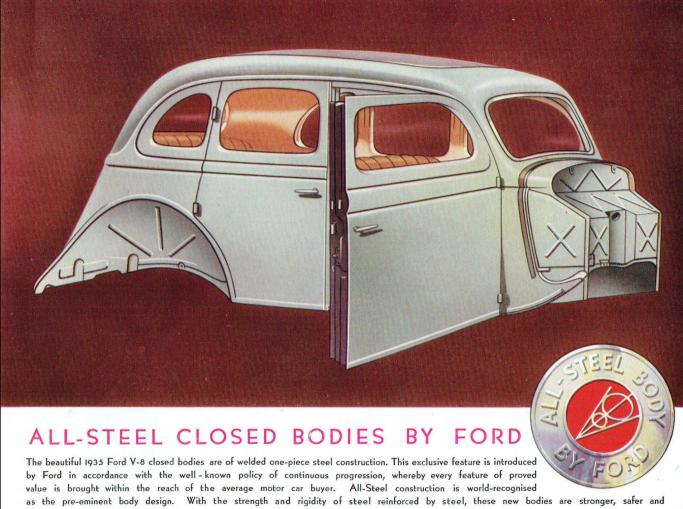
as the pre-eminent body design. With the strength and rigidity of steel reinforced by steel, these new bodies are stronger, safer and silent. They have longer life than any other type of body and the original perfect fitting of doors is retained permanently. Because of welded steel joints, the causes of squeaks and body noises are eliminated. There is no substitute for the quality of an All-Steel body.
